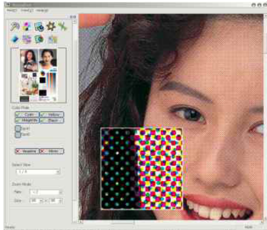
Analysis of halftone pattern with partial zooming tool
