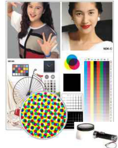
Hardproofing of halftone on inkjet output
